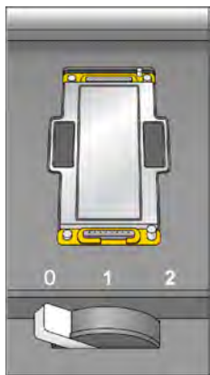
Figure 28 Flow Cell Lever in Position 0
