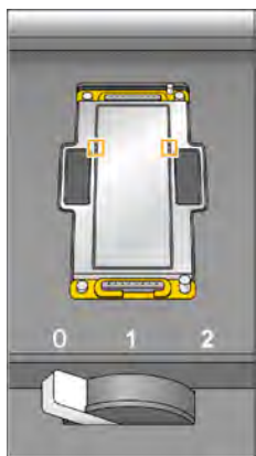
Figure 22 Inspect Vacuum Holes
