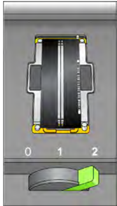
Figure 32 Flow Cell Lever in Position 2
