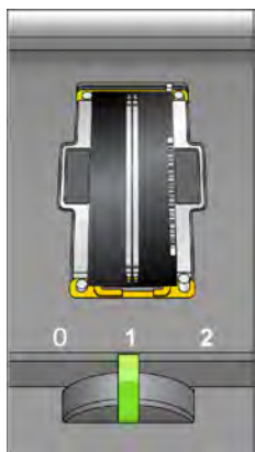
Figure 33 Flow Cell Lever in Position 1
