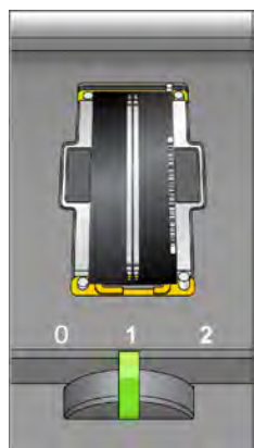
Figure 31 Flow Cell Lever in Position 1
