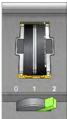
Figure 38 Flow Cell Lever in Position 2
