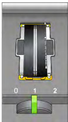
Figure 37 Flow Cell Lever in Position 1
