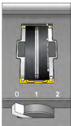
Figure 34 Flow Cell Lever in Position 0
